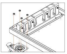
Assemble castors onto frame and holder.
