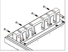
Screw the holder components together.
